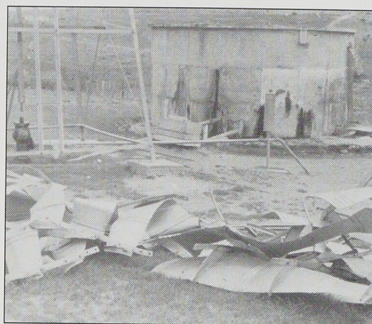
Broken head gear from a windmill lies beside a storage tank. The tank, fed by another windmill downhill, is overflowing because it relies on this windmill to pump the water to a second tank further uphill. People living near the empty upper tank have to walk to collect the water they need.
