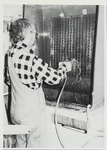
4) Joe Tilson washing the acid off a cop per plate after etching in acid has been completed
