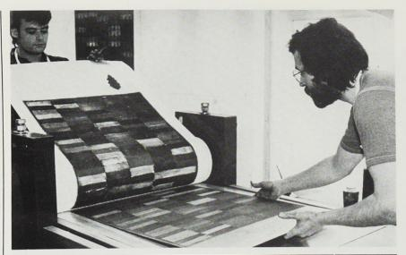
6) Paper trapped to allow changing of colour plate for line plate in the making of Oak Mantra
